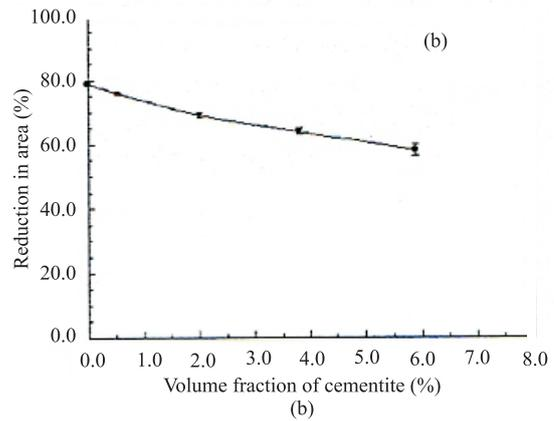
Fig.10. (a)Percentage reduction of area with different microstructures, and (b)Reduction of area under different volume of 2<sup>nd</sup> phase.
