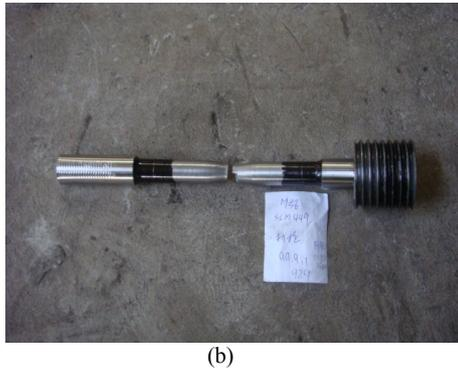
Fig.9. (a)A machined test-piece in ISO 898.1 specification, and (b)A machined test-piece from stud.
