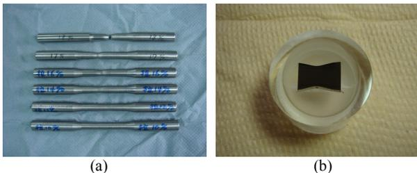
**Fig.11.** (a) Test-pieces with different elongation %, and (b) Metallurgical sample of 17% testpiece.
