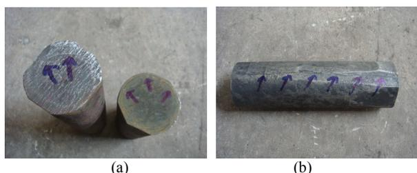
**Fig.8.** (a)Circular quench cracks, and (b)A longitudinal quench crack.
