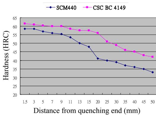
Fig.4. Jominy end-quench test result of SCM440 and BC 4149.
