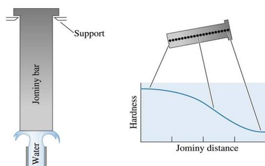
**Fig. 2.** The Jominy end-quench test.
