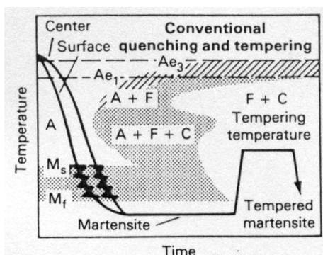
**Fig.3.** Quench and temper sequence.
